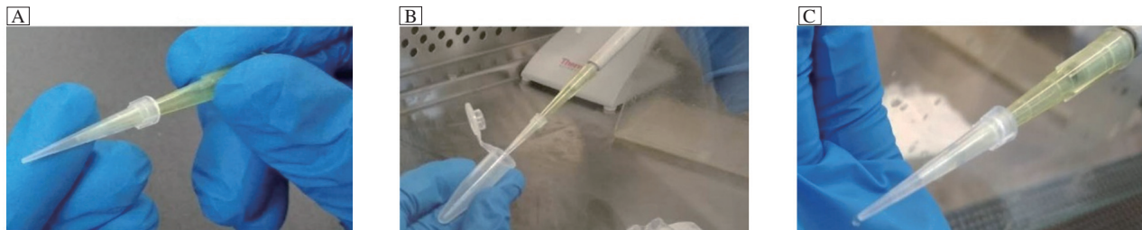
Fig. 1 The construction of the tip complex. (A) The insertion of a 200 µL tip into a 10 µL tip. (B) Using a 20 µL pipette to connect to the above and insert into the microcentrifuge tube without pressing the pipette. (C) After removal, and pressing the pipette.
