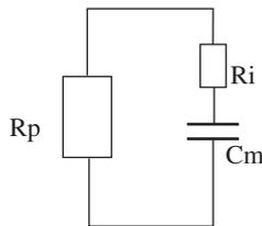
**Fig. 1** Equivalent circuit of the red blood cells. It consists of  $R_p$  (plasma resistance) in parallel with a series circuit given by  $R_i$  (resistance of cell interior) and  $C_m$  (membrane capacitance).
